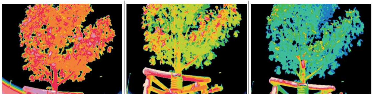
Figure 2: Thermal imaging camera images before rotation (left), during rotation (centre), and after rotation (right). High surface temperatures are represented by red-coloured areas and lower surface temperatures by blue areas [Henninger 2020, p. 76].
