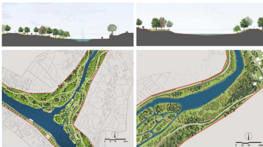
Design of green embankments, riparian landscape and rehabilitated wetlands with increased flow capacity and enhanced biodiversity. Source: ADB consultants for Asian Development Bank.
